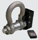
The shackle dynamometer SHS-BT is designed to endure particularly demanding industrial use. With its compact structure, the device fits perfectly into small spaces, which makes it excellently suited for use in the field. Available capacities range from 20 tonnes up to 120 tonnes.
