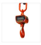
The Tamtron PCS crane scale is designed especially for lighter industrial weighing for loads of under 10,000 kg. The crane scale is light, which allows it to be moved effortlessly as required. The scale is controlled by a remote control device, which facilitates safe working. The weighing information
